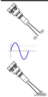
Electronics of LSV excites the piezo-electric- crystals inside the tuning fork, which makes the fork tines vibrate at their natural resonance frequency in free air.
